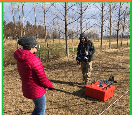
Ground penetrating radar being pulled over soil to determine soil properties.
