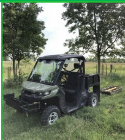
UTV pulling the electrical conductivity sensor in a sled to detect changes for evaluating soil moisture at a silvopasture research site near Fayetteville, AR.
